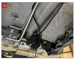
O) Underneath the car using a 10mm socket remove the nuts that hold the plastic box to the car and gently pull it down, you don't need to fully remove it, this is where you fed the wire to in a previous step.
