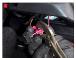
J) Use a tool such as adjustable grips or pliers to drive the metal connector into the Scotch lock to ensure good connection.
